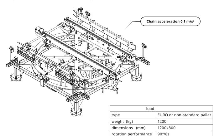
The control system ensures precise rotation adjustment, enabling 360-degree manipulation and changing the direction and orientation of the goods. Thanks to the device, the transportation process becomes smoother and more efficient.
