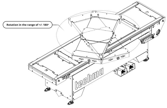
The manual turntable allows the operator to lift the material above the roller conveyor, eliminating the need for heavy lifting. This significantly reduces the risk of injuries and body strain while increasing the comfort and safety of work. The operator can freely perform manual tasks and easily rotate the material without the need for relocation.
