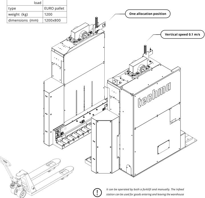
station can be used for goods entering and leaving the warehouse (e.g., empty cartons). It is equipped with a control gate that signals oversize pallet loading.
