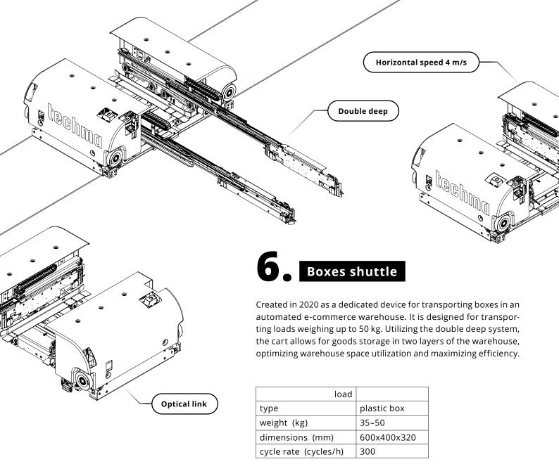
It stands out for its **high operating speed and low noise level**, making the work environment in the warehouse more comfortable.
